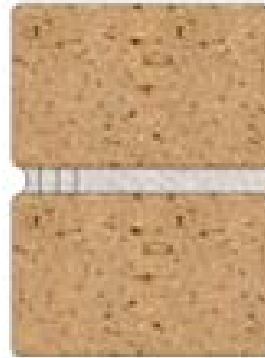
FINAL PASS TOOLED TO CONCAVE OR VEE PROFILE TO MATCH EXISTING
