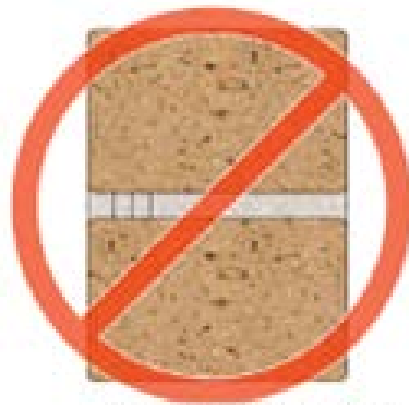
FINAL PASS INCORRECTLY SMEARED ABOUT BRICK EDGES RESULTS IN EXAG- GERATED JOINT WIDTH
